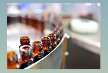
ENERGY COSTS DROP 2-3% FOR EVERY 10% CULLET USED IN THE MANUFACTURING PROCESS VIRGIN MATERIAL FROM WY MELTS AT 3000, CULLET MELTS AT 1500
